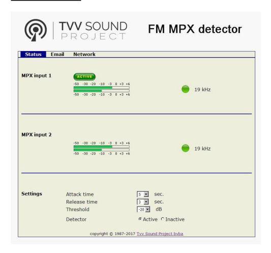
The top half of the page shows the status of the 2 connected sources: MPX input1 and MPX input2. Input 1 is the main source and will always be connected to the output if this signal is on. This is visible by the text ACTIVE. The meter (s) can see if there is a signal. With each input there is also a signal for the 19Khz. If present, the signal is green, in the absence of red. In the bottom half, Settings have a number of settings.
